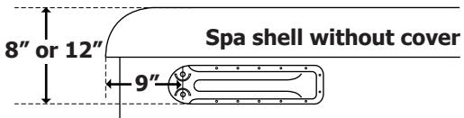
By positioning the Mounting Brackets 8" down from the top of the spa shell, approximately 9" clearance behind the spa will be needed. Mounted at this position, approx. 75% of the spa cover will be standing above the spa surface in the off position. By positioning the Mounting Brackets 12" down from the top of the spa shell, approx. 15" clearance behind the spa will be needed. Mounted at this position, approx. 50% of the spa cover will be standing above the spa surface in the off position.
