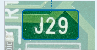
J29 is a heater disable switch input.
